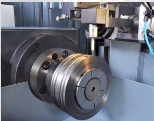
Work Holding arrangement & Probe for centering
